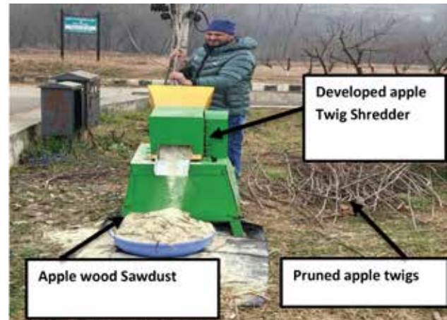
Fig. 4. Working view of the developed apple twig shredder at a high density apple farm.
