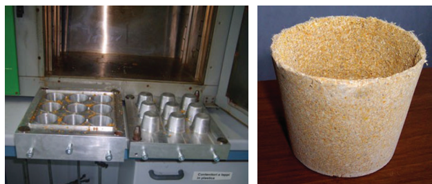
Fig. 5. Molds and casting biodegradable nursery plant pots. (Courtesy: Santagata et al. , 38).
