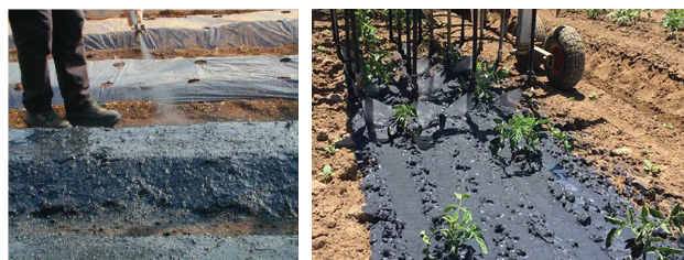
Fig. 4. Application of sprayable biodegradable polymer membrane shortly after spraying and polymer treatment plots. (Courtesy: Santagata et al. , 38).
