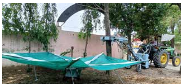
Fig. 1. A view of the developed tractor-operated tree shaker mounted on the Jamun tree along with the collection unit
