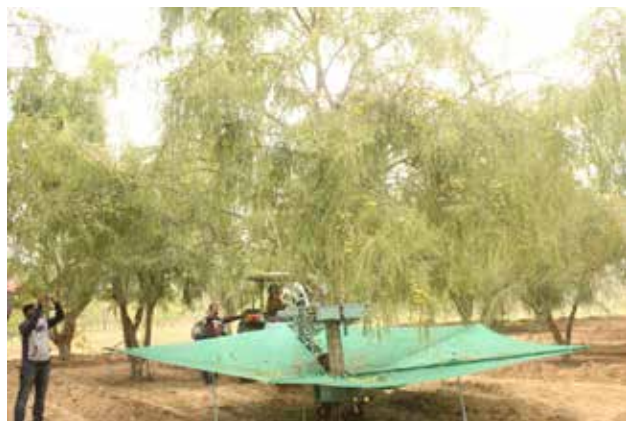
Fig. 2. A view of developed tractor-operated tree shaker harvesting Aonla fruit
